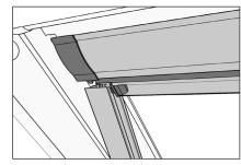
Slide fabric into the front channel of the siderail.
