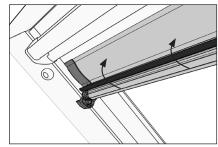
Pull handle away from the window and fold upwards against the front of the cassette.
