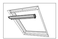
Position the cassette at the top of the window frame and press firmly.
