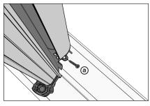
Secure the cassette using screw (a).
